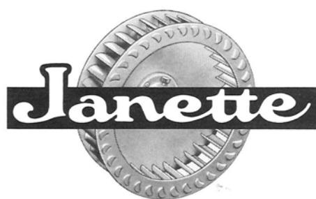
These components are designed for wheels ranging from  $7\frac{1}{16}$ " to 15" diameter and  $2\frac{3}{4}$ " to  $5\frac{1}{2}$ " wide. Heavy 16 ga. steel construction is standard, however, they are available in stainless steel and aluminum. The housings are universal so they can be used for either rotation in eight positions. All parts are primed and bolt together for easy assembly.
